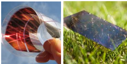
Figure 6-14 Plastic Solar Cell films developed by Georgia Tech's Bernard Kippelen allows the flexibility of use of solar energy generation within the balcony setting as an added screen. This film with adopted shape memory polymers can allow it to react to different angles of the sun to increase efficiency.
