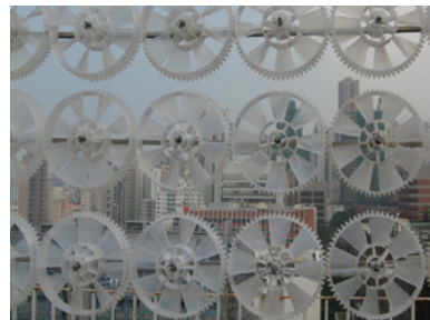
Figure 6-7 Micro Wind Turbines developed at Hong Kong University have a compact 25 cm rotor diameter and can be aligned in series to generate energy with low winds. This technology makes it ideal for use in urban
