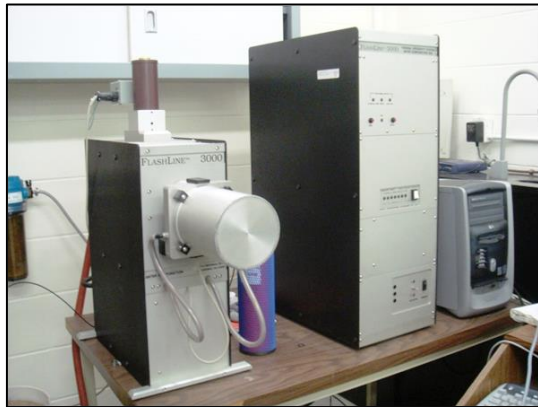
Figure 4-7 Flash Line 3000 (left) and Flash method (right) 58
