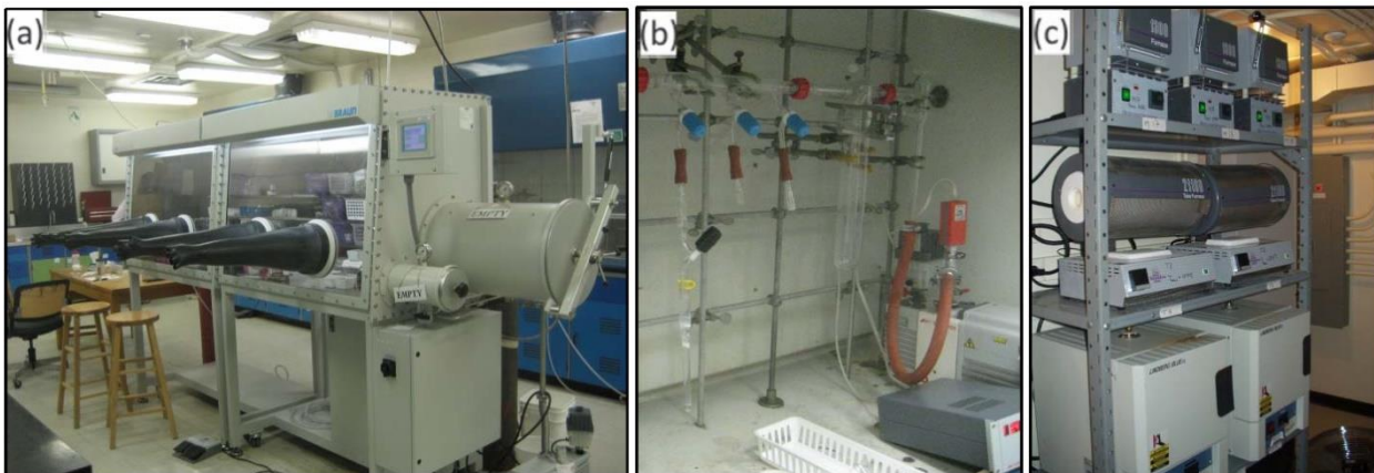
Figure 3-1 (a) Argon-filled glove box (b) Vacuum line (c) Manual furnace (top) Programmable furnace (bottom)
