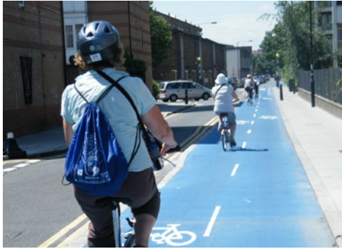
Figure 3-13 Typical cycle track
