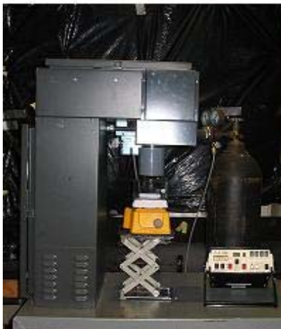
Figure 3.1 Collimated Beam Apparatus (Calgon Carbon Corporation, Pittsburgh)
