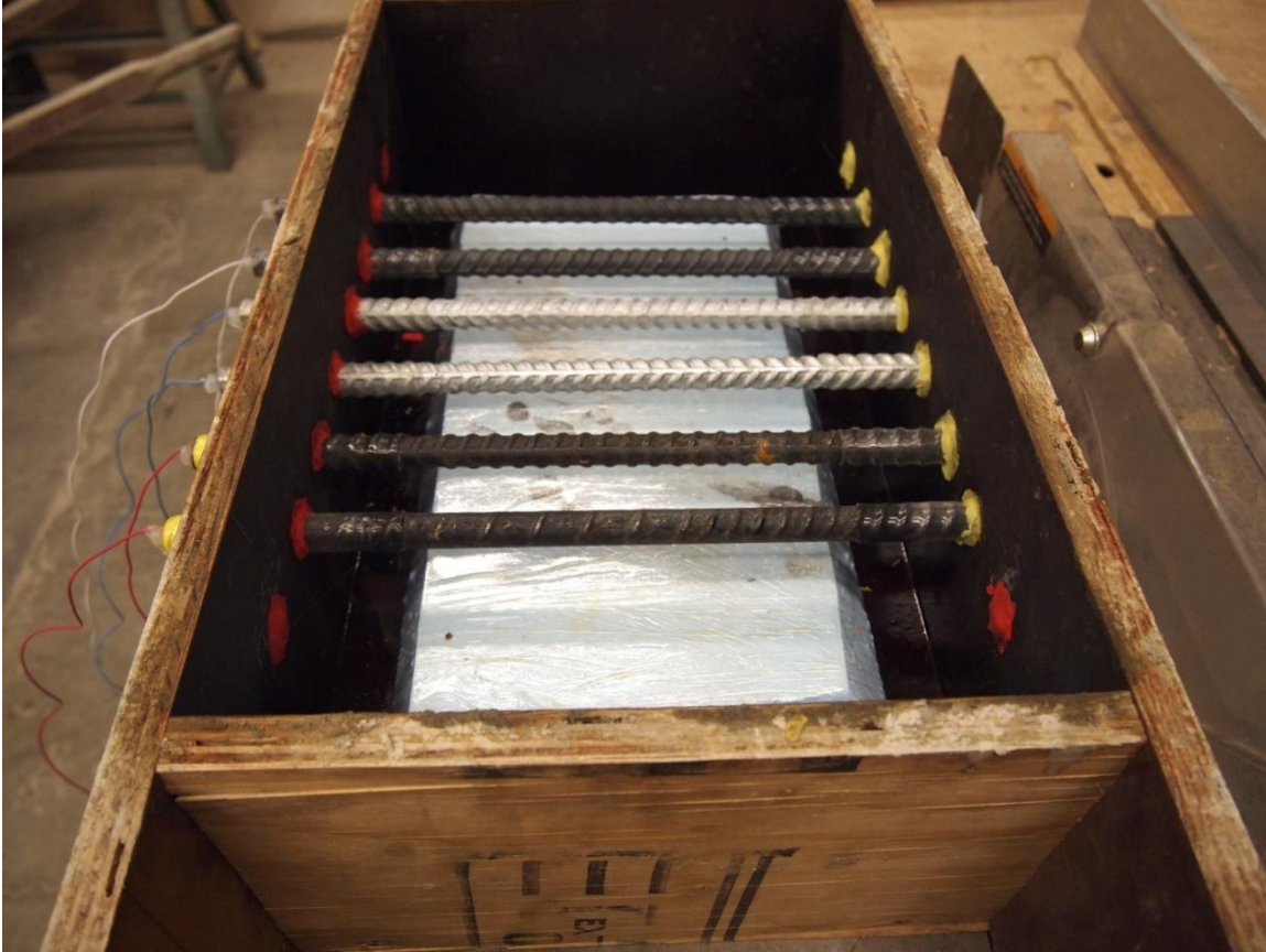
Figure 3-4: Sound concrete formwork
