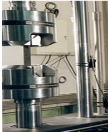
Figure 4.9. The experimental setup for material fatigue testing.
