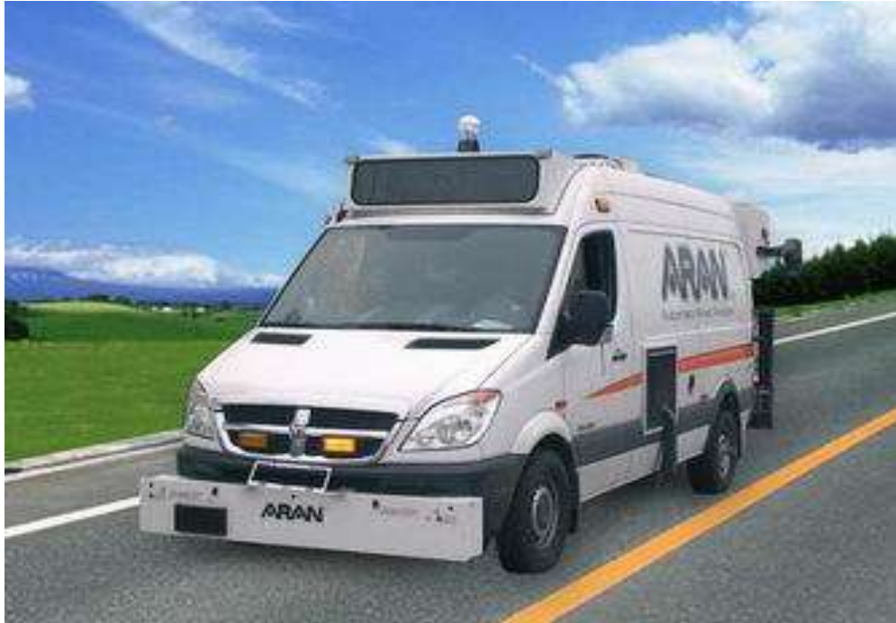
Figure 3-1: ARAN Automatic Road Analyzer ( www.epc.com.hk )
