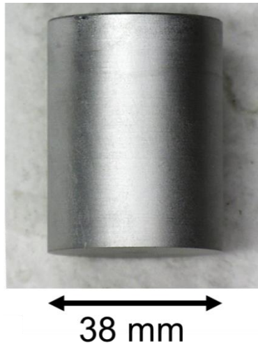
Figure 3-12 – Macro photo of a prepared AA3003 sample prior to immersion testing.
