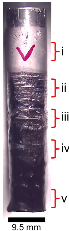
Figure 6-8 – Resulting sample surface after test immersion. Al-1Mn-0.0008Mg sample immersed in Al-10Si-0.0008Mg melt at 913 K (640 °C). Calculated oxide thickness on sample prior to immersion in the melt was 28 nm.
