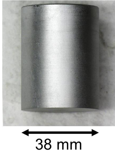
Figure 5-2 – Photo of a prepared AA3003 sample prior to immersion testing.
