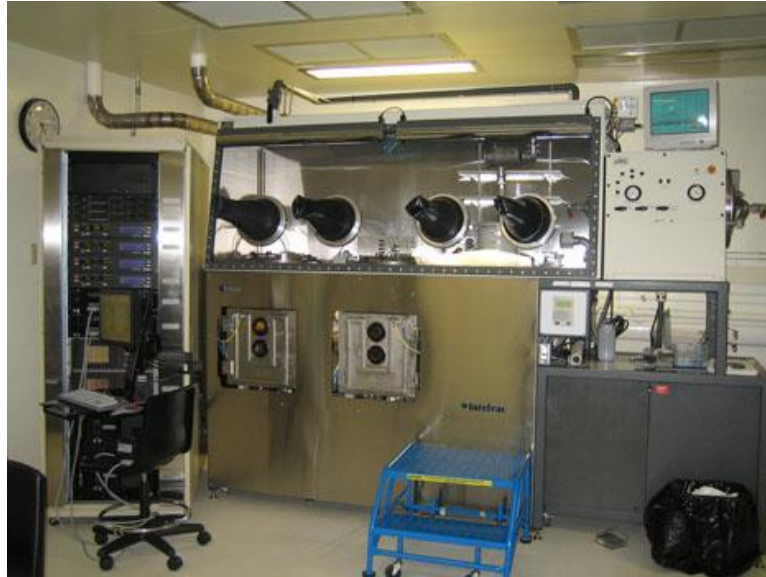
Figure 2.1.5: Intlvac Thermal/E-beam Evaporator (left and right chambers, respectively), with a nitrogen glove box above[24]. After samples are loaded the chambers are pumped to a low vacuum, and the same is exposed to a plume of ejected material instigated by Joule heating or e-beam exposure, respectively.
