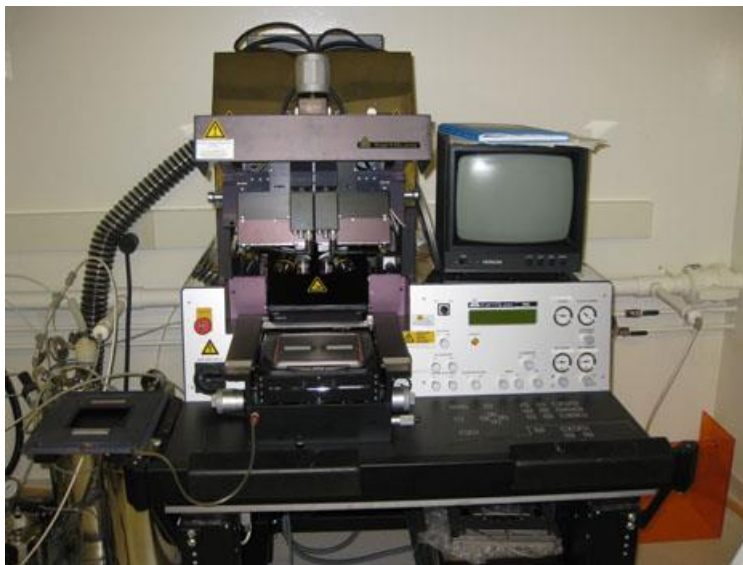
Figure 2.1.2: Karl Suss MA6 Mask Aligner[24]. A sample is aligned with a glass plate bearing the mask pattern (written in Cr here), and exposed with a UV lamp to selectively expose the photoresist with the mask pattern.
