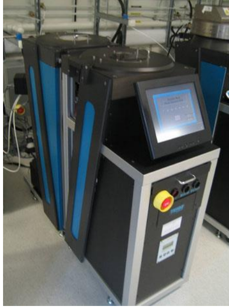
Figure 2.1.1: Phantom II RIE system[24]. A hybrid physical-chemical etching system, RIE is simultaneously capable of some material selectivity and an anisotropic etch progression.
