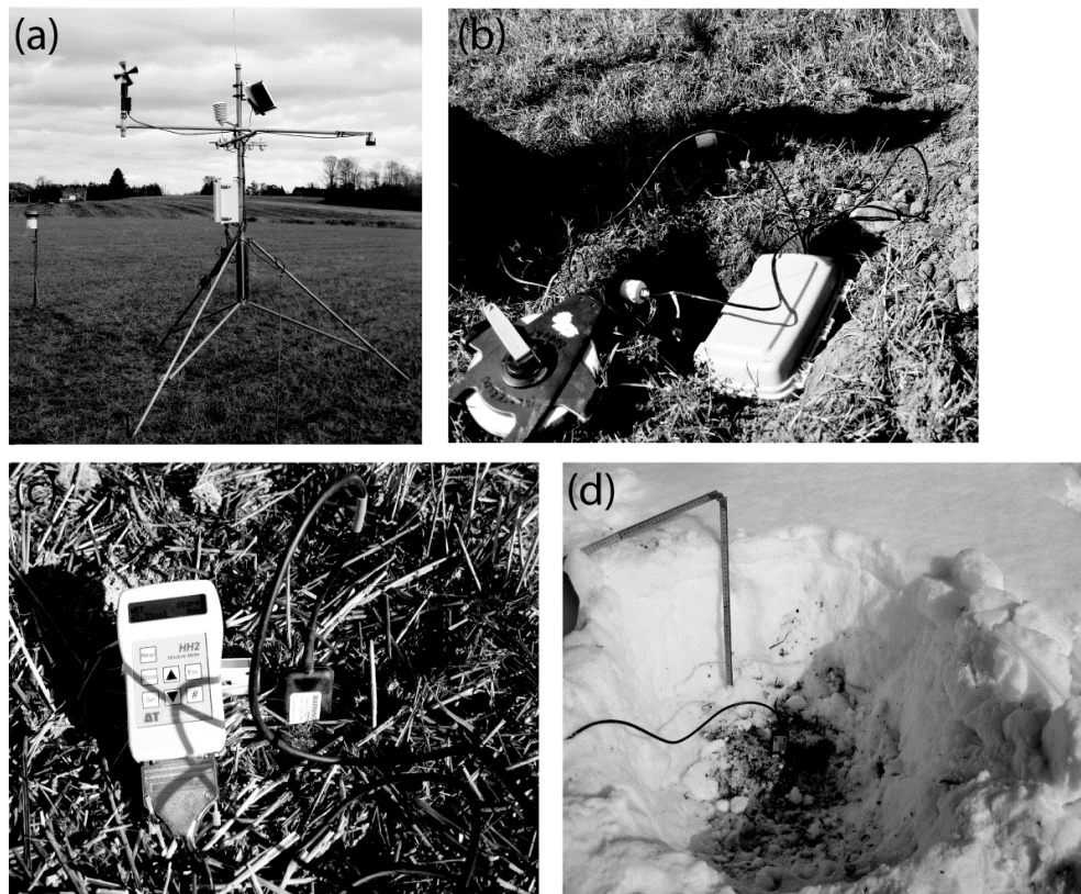
Figure 3.3 (a) Weather station; (b) Hydra probes installed to provide soil measurements at two depths: 5 cm and 15 cm; (c) Delta-T WET sensor used to collect soil measurements across the entire study site; (d) soil moisture and snow depth measurements were made during the winter.
