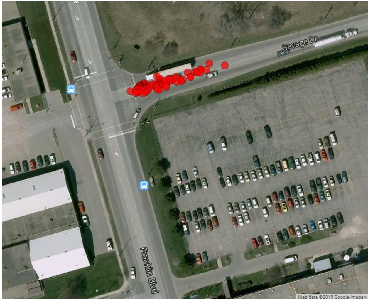
Figure E-3: Unscheduled Stop Observations for Franklin at Savage Dr.
