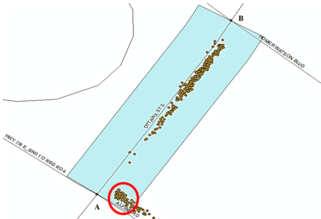
Figure 2-7: Invalid Stopped Delay Observations Captured by the Buffer Zone in the ArcGIS
