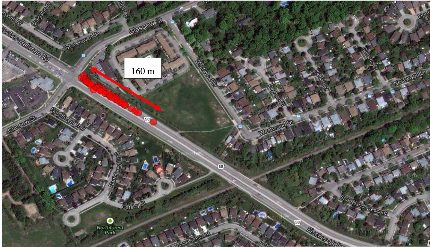
Figure C-20: The unscheduled stop observations superimposed on Google Maps for Fischer-Hallman at Glasgow Intersection
