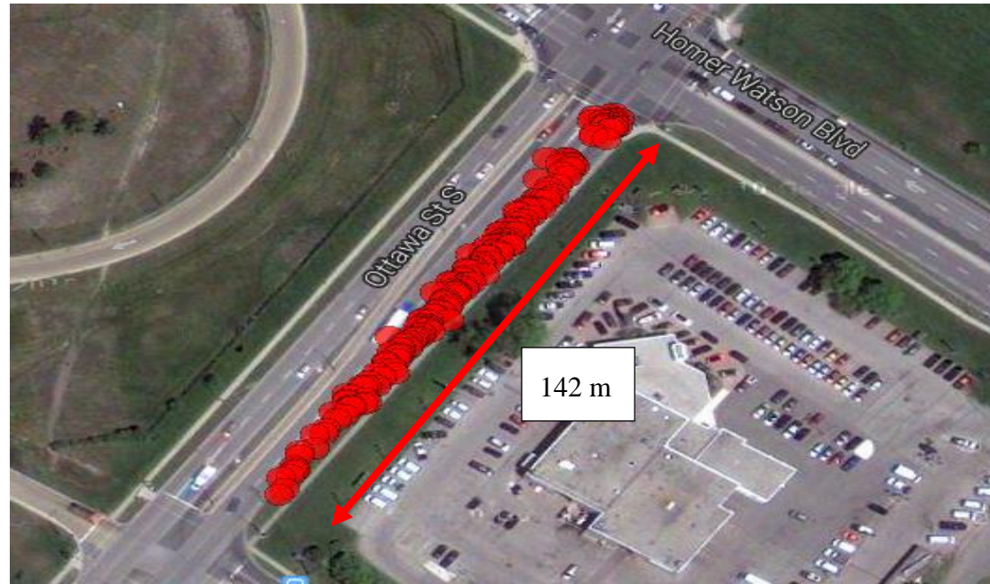
Figure C-12: The unscheduled stop observations superimposed on Google Maps for Homer Watson at Ottawa intersection In Figure C-11(B) the observations from adjacent segments are excluded from the analysis.
