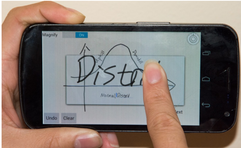
Figure 1.2: InkAnchor allows users to easily create ink-based notes on a touchscreen mobile phone. In this case, the user is annotating a function image with texts in different directions.
