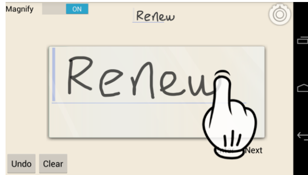
Figure 3.4: A user can write on the glass screen, and the ink will be scaled down automatically and show up on the background in real time.
