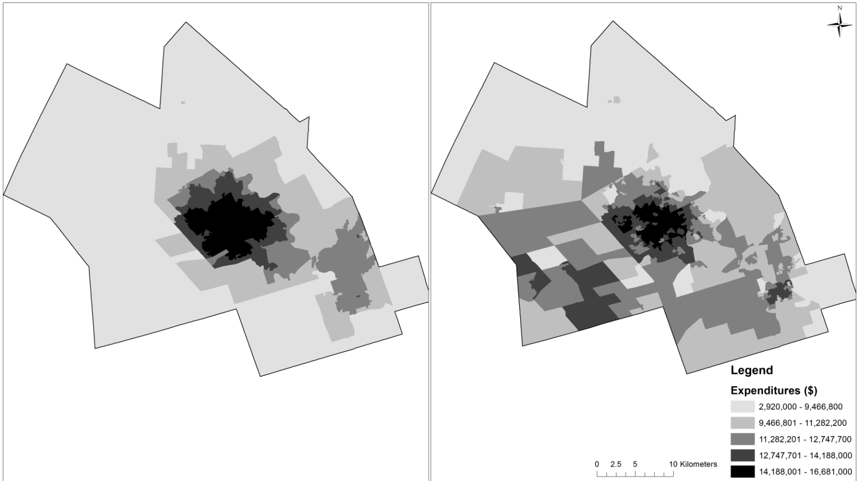
Figure 3.6: Huff's model expenditures for Euclidean distance- (left) and network-based (right) spatial interaction costs.
