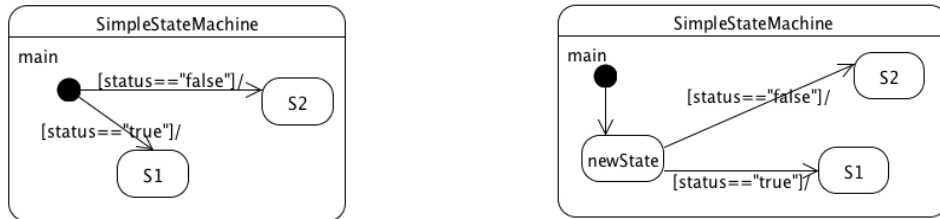
(a) Labeling on arrow from a pseudo state to a default initial state is not allowed; more than one arrow from a pseudo state is also not allowed. (b) If user needs to use guard condition on the arrow from a pseudo state, user can redefine the original pseudo state as a new default initial state.
