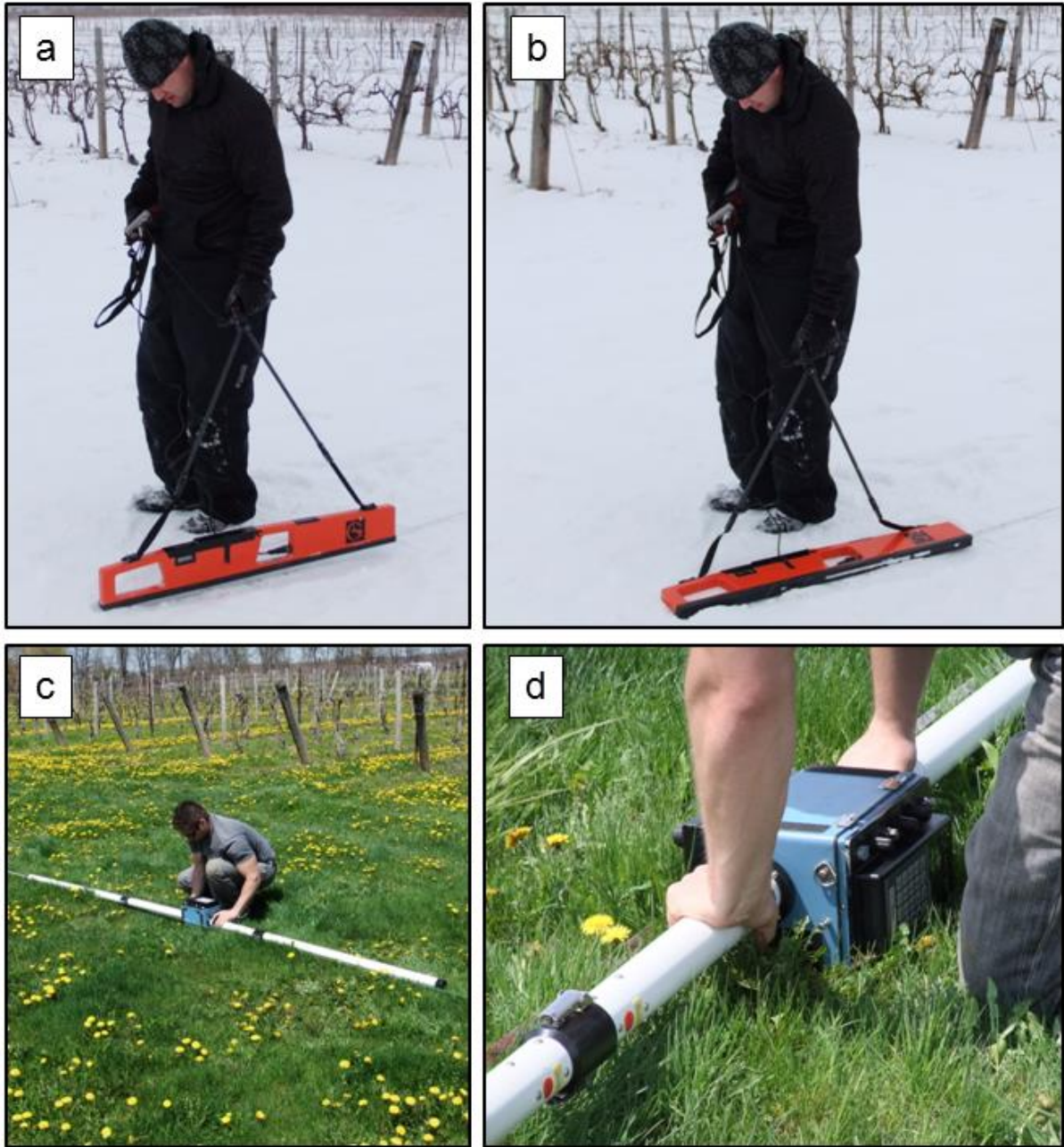
Figure 5.2 – Examples of EMI data acquisition using the EM38 and EM31 in both vertical and horizontal dipole orientations. a) EM38 vertical dipole, b) EM38 horizontal dipole, c) EM31 vertical dipole, d) EM31 horizontal dipole.
