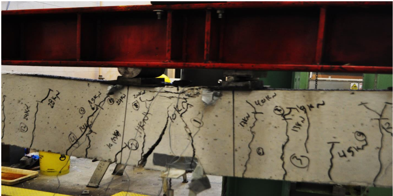
Figure 4- 4 Mode of failure of a non-prestressed beam
