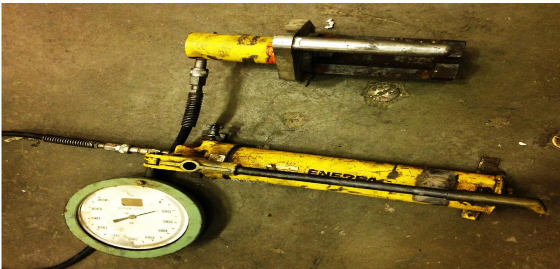
Figure 3- 7 Hydraulic manual pump and jack used in pre-seating the anchor
