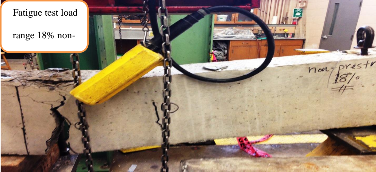
Figure 6- 1 Mode of failure of non-prestressed beam under fatigue load (load range 18%)
