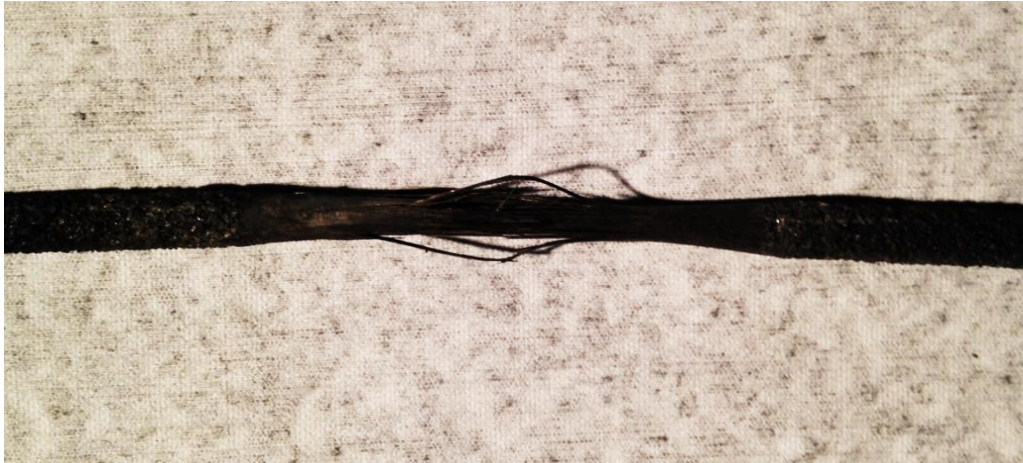
Figure 5- 1 Rupture of tested basalt bars under axial fatigue test
