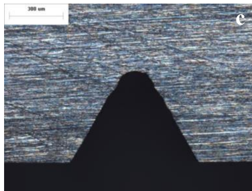
Figure 7-2(a) Schematic drawing of the DENT specimens (ND and TD) and the corresponding dimensions; The sheet (RD-TD-ND) and specimen (L-W-B) coordinate systems are defined. Note that in ND specimens: L \parallel RD, W \parallel ND, B \parallel TD and in TD specimens: L \parallel RD, B \parallel ND, W \parallel TD . (b) Typical DENT (ND and TD) specimens; (c) Notch appearance from cross sectional view (notch depth: 0.5 mm)
