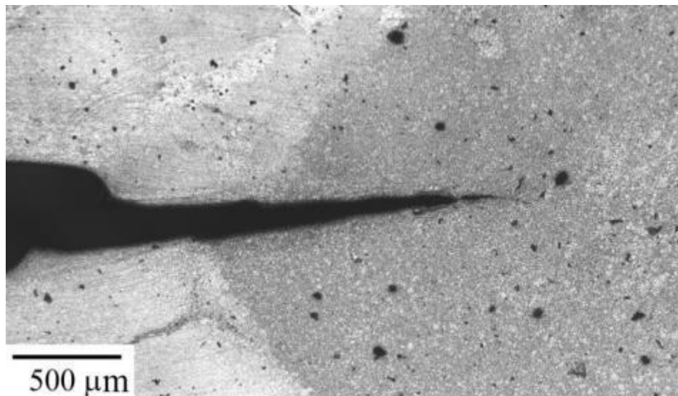
Figure 6-11 Failure in ZEK100/ZEK100 weld in as welded condition
