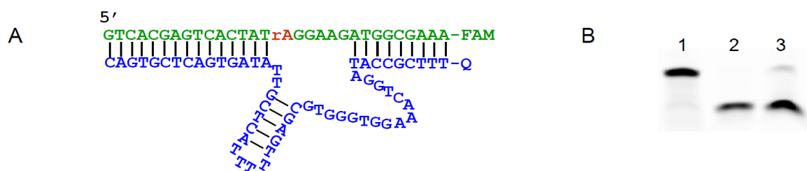
Figure 2.13 Design of the fluorescent Ce13d DNAzyme beacon. A) The sequence of the DNAzyme beacon. B) Confirmation of cleavage in the catalytic DNA beacon based sensor.
