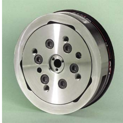
Figure 5.3: Force/Torque sensor Delta IP60 from ATI Industrial Automation[39].
