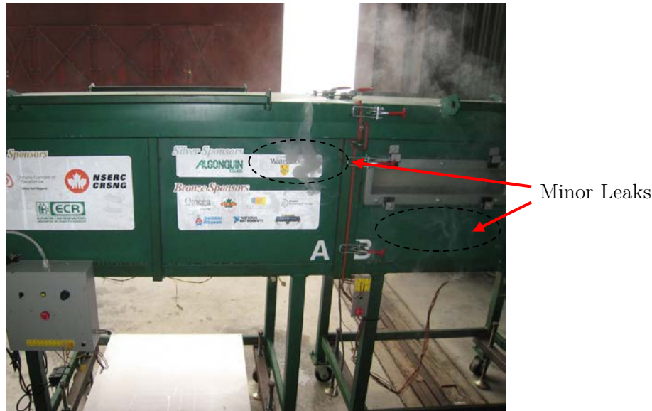
Figure 4.4: Air leak test after the tunnel repairs
