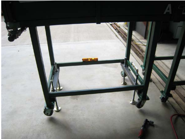
Figure A.6: Final height adjustments are made to level the tunnel sections even
