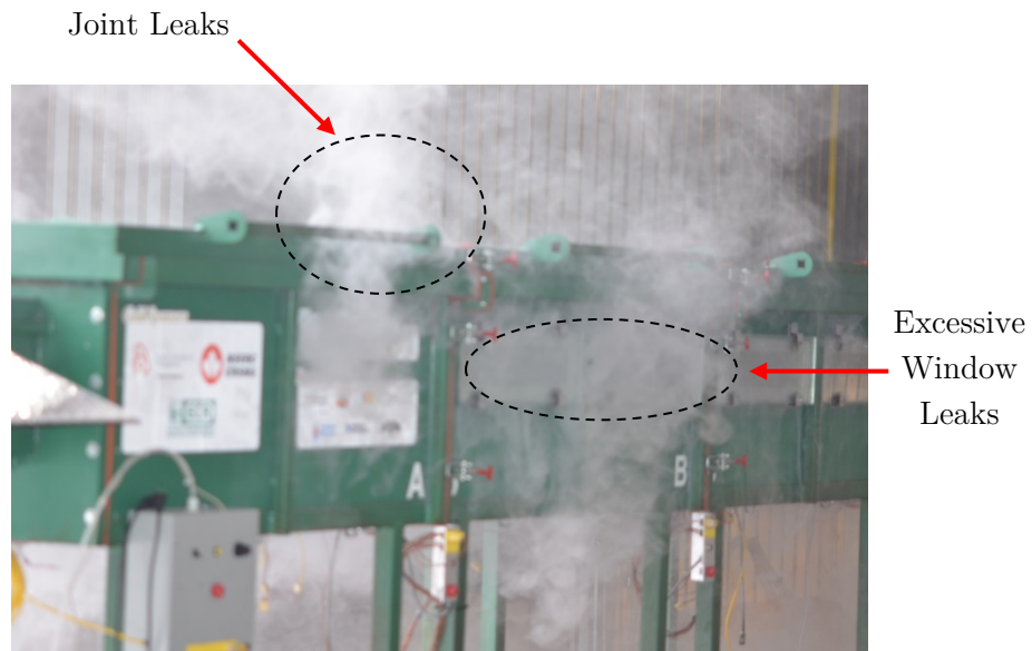
Figure 4.2: Photograph of the air leak test, window view of the tunnel
