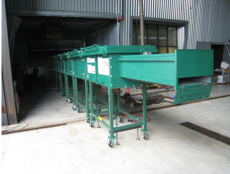
Figure A.10: Every module is accommodated with a corresponding lid assembly to conceal the tunnel
