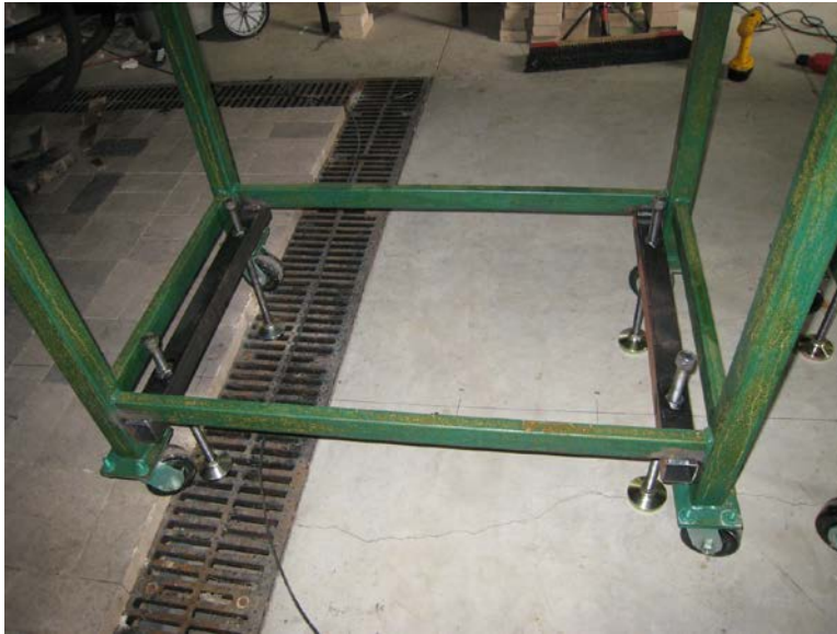
Figure A.4: Height adjustment rods are lifted to align the height between the exhaust and the tunnel opening
