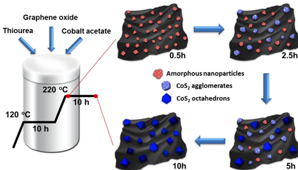
Figure 7-9: Proposed growth schematic of \text{CoS}_2 octahedron nanoparticles supported on nitrogen and sulfur doped graphene. Reproduced in adapted form from 253 , with permission of the Royal Society of Chemistry.
