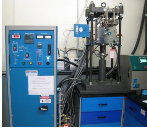
Figure 16: FR-210-30T hot press by Oxy-Gon Industries
