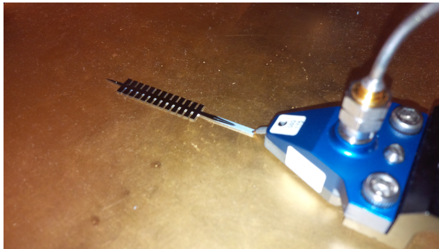
Figure 3.51: A fabricated sample of the proposed CPW-fed side grating antenna.
