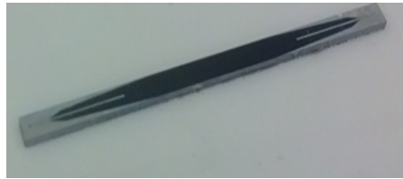
Figure 5.12: Picture of the fabricated back-to-back test structure optating at the W-band.
