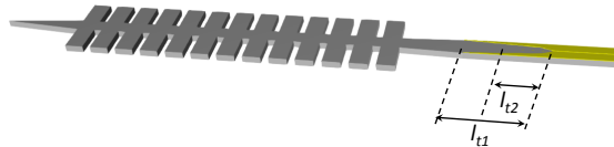
Figure 5.15: 3D model of the proposed CPW-fed side grating antenna.
