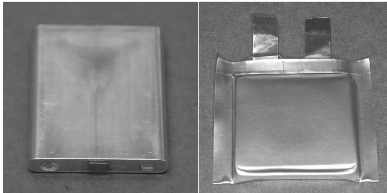
Figure 17: Examples of prismatic cell hard case (left) and pouch (right) [36]
