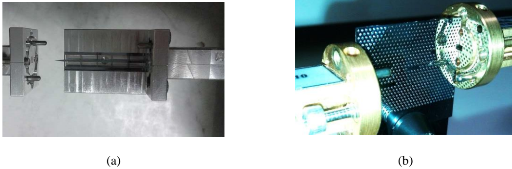
Fig. 2.5 a) Test setup of the high-resistivity Si rod dielectric waveguide [69] and b) test setup of the photonic crystal resonator devices mounted between two metallic ports [71].
