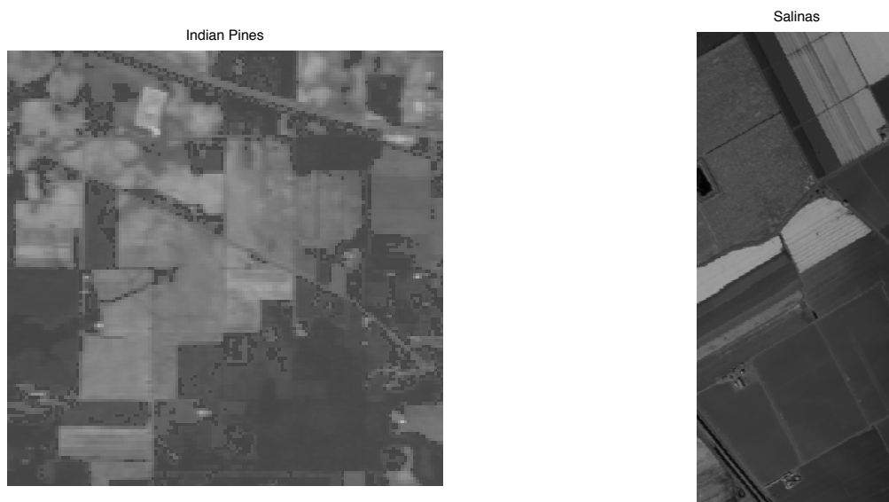
Figure 4.5: The image on the left is the band number 23 of the hyperspectral image Indian Pines. The image on the right corresponds to band number 57 of the hyperspectral image Salinas.
