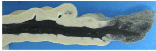
Figure 2-9. Fluid-fracture cross-section indicating more active leak-off at fracture tip (Germanovich et al., 2012).
