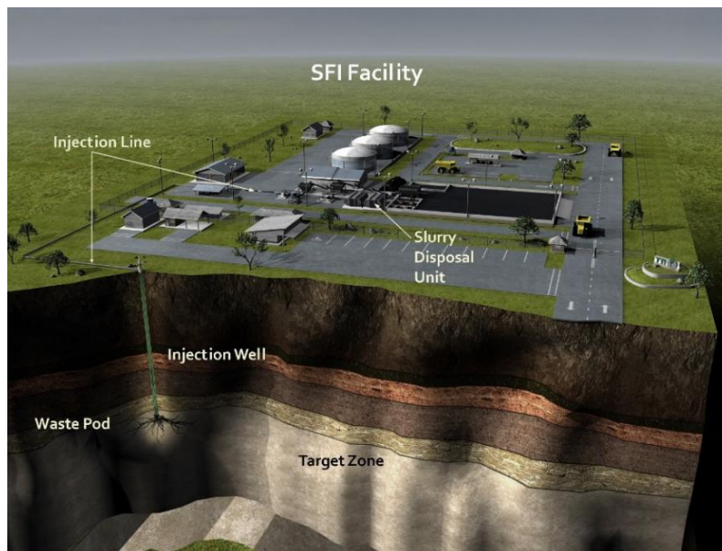
Figure 1-3. A schematic of SFI facility and operation (courtesy of Terralog Technologies Inc.).
