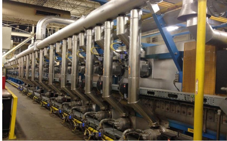
Figure 3: Roller hearth furnace located at Formet Industries.
