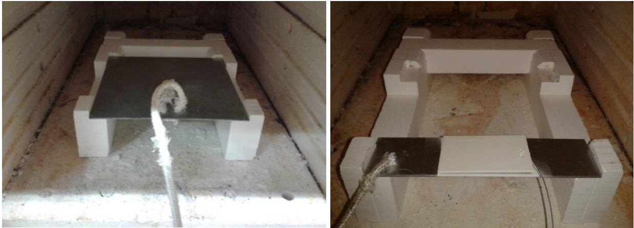
Figure 9: Setup for thermocouple measurements conducted in the muffle furnace on unpatched blanks (left) patched blank (right).
