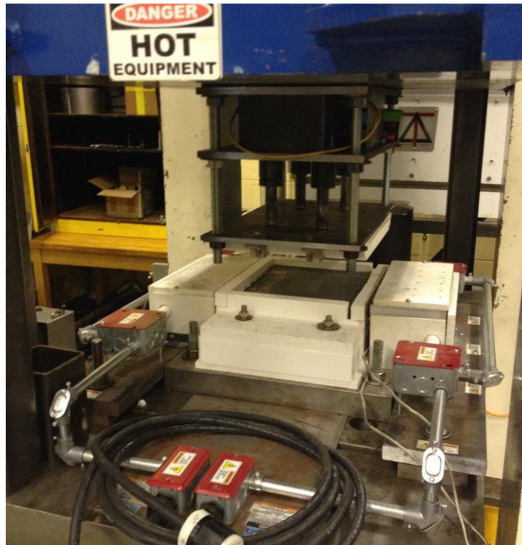
Figure 18 - Final die set assembly mounted in the 250 ton hydraulic press.
