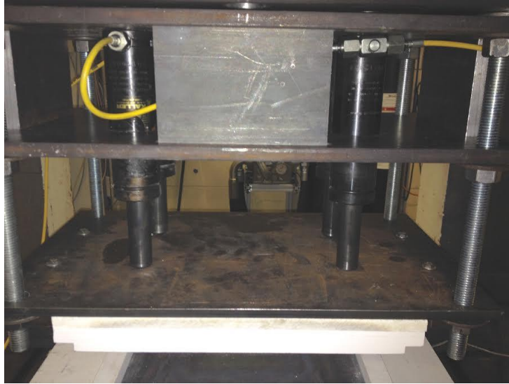
Figure 17 - Upper striking surface with primed nitrogen springs.
