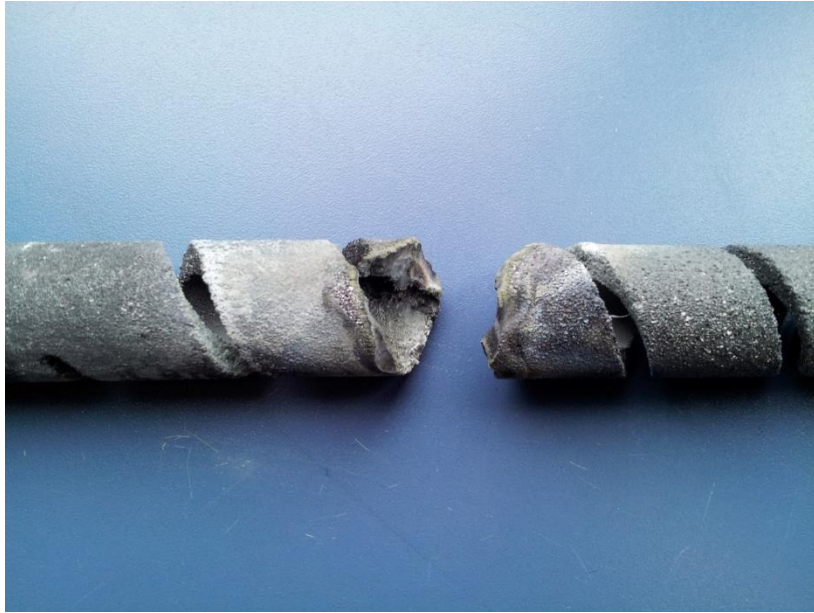
Figure 25 - Fractured heating element caused by the application of stress during non-uniform thermal expansion of the monolith.
