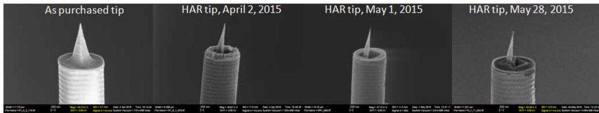
Figure 5.27. High aspect ratio tips processed out of Rocket tip at different times to show reproducibility.
