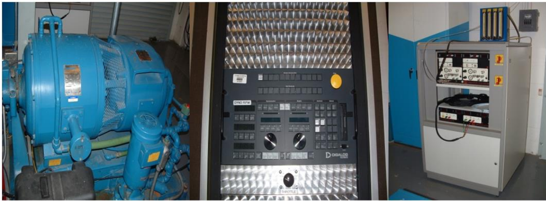
Figure 3-2 Test equipment: a) dynamometer, b) external Panel and c) FID hydrocarbon analyzer
