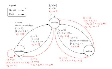
Figure 2.6: Repaired automaton of the TAD in Fig. 2.1
