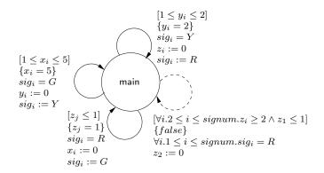
Figure 2.7: Automaton for traffic controller *i*.
