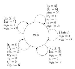
Figure 2.8: Automaton for train signal controller
