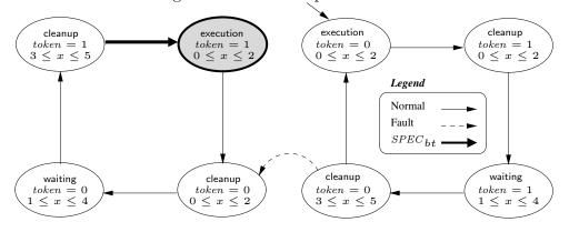
Figure 2.3: Zone graph of the timed automaton in Fig. 2.1
