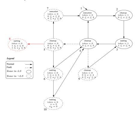
Figure 2.4: Synthesized zone graph of the timed automaton in Fig. 2.1
