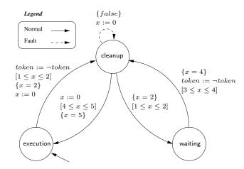
Figure 2.1: A timed automaton with deadline augmented with one fault switch
