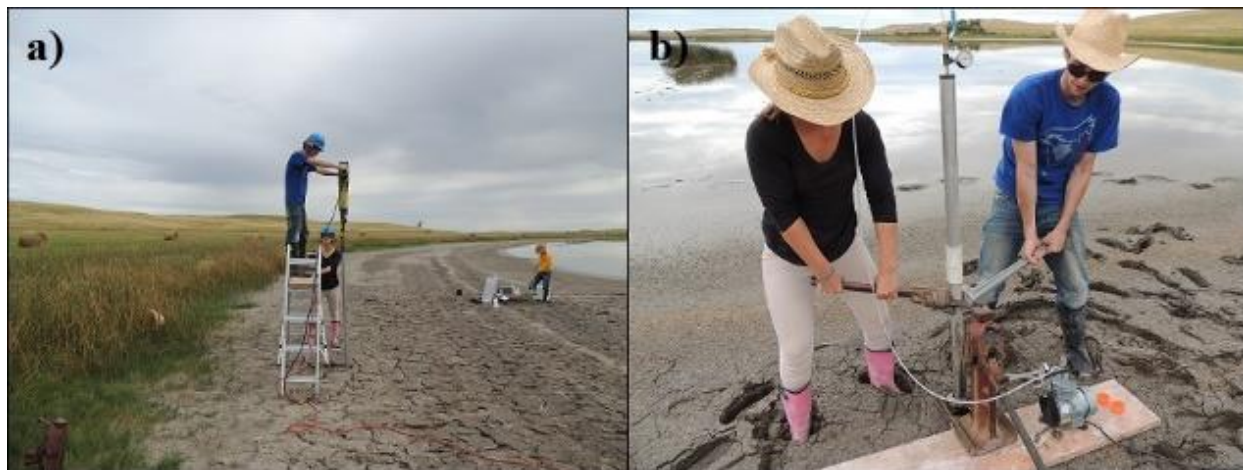
Figure 16. Sediment core sampling in the 2014 sampling year, showing a) inserting core into ground using a jack hammer, and b) the removal of the core using a vacuum suction pump and a railway jack.
