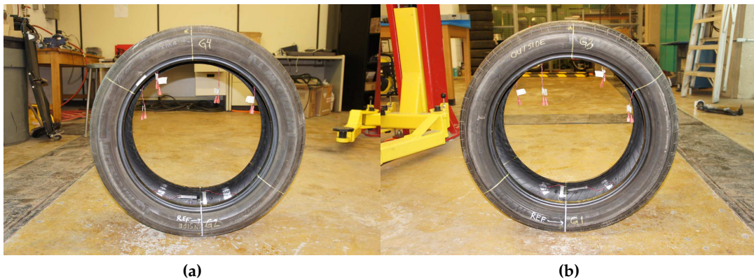
Figure 5.31 – Instrumented Tire for Smart Tire Revision 2: (a) Inside (b) Outside
