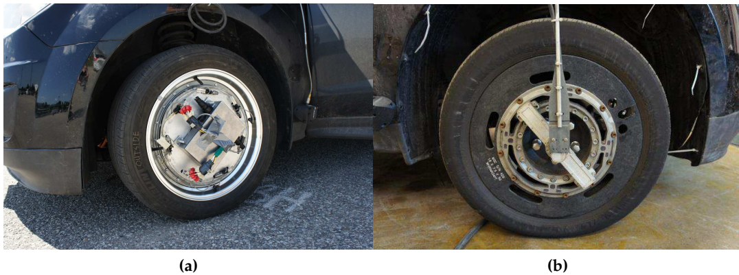
Figure 5.11 – Research Vehicle Front Corners: (a) Left Front with Smart Tire Revision 1 (b) Right Front with Wheel Load Transducer
