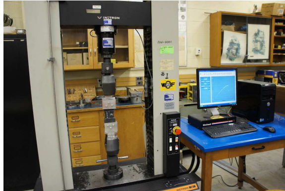
Figure 3.6 – Instron Machine with Tire Sample
