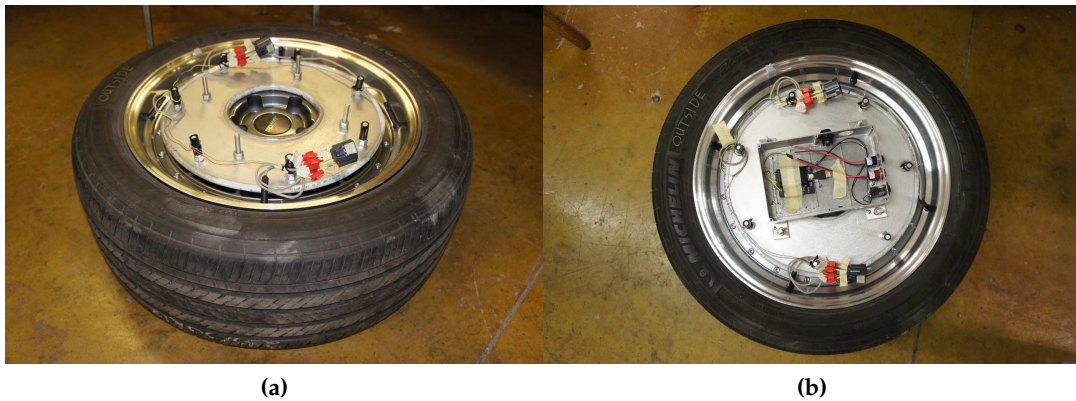
Figure 5.6 – Smart Tire Prototype Revision 1: (a) Without Data Acquisition Box (b) With Bottom Part of Data Acquisition Box Housing
