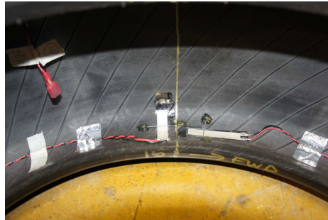
Figure 5.32 – Detail of Sidewall Sensor Pair in Smart Tire Revision 2
