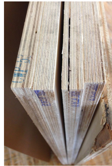
Figure 109: From left - 3/4" Asian plywood, 3/4" Baltic birch plywood, 1/4" construction-grade plywood
