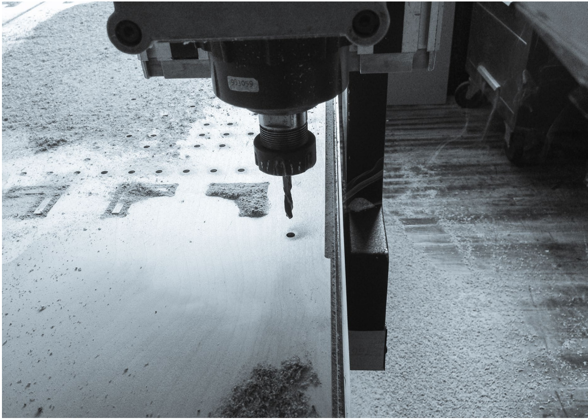
Figure 130: Smoke from the flat end mill bit drilled into the spoil board for pins to enable rotation of the 6' parts. Future parts used a drill bit to prevent this.
