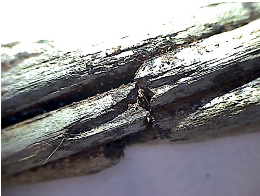
Figure 5-14 – Failure at a corrosion pit location on a wire specimen
