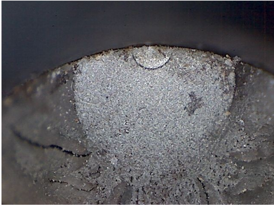
Figure 5-12 – 200× magnification of a sample the fretting damage
