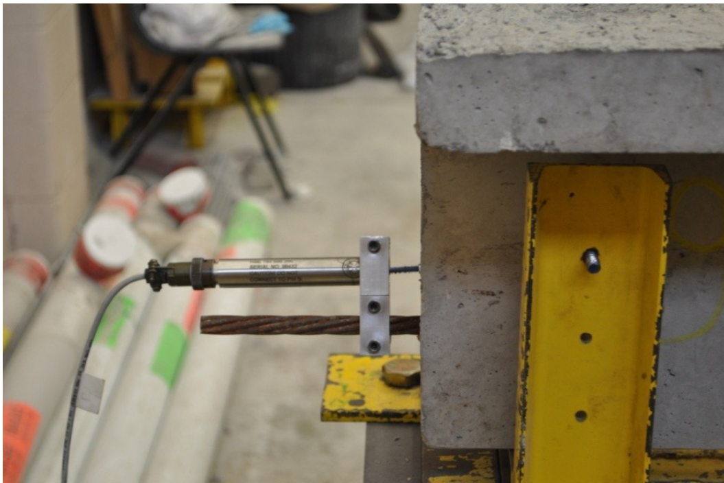
Figure 4-14 – LVDT mounted at beam end to monitor end slip of prestressing strand
