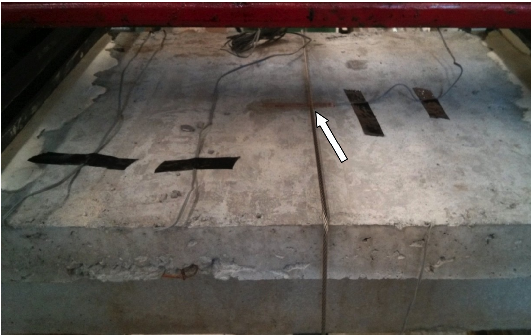
Figure 3-15 – 60 mm strain gauge to monitor the concrete compressive strain
