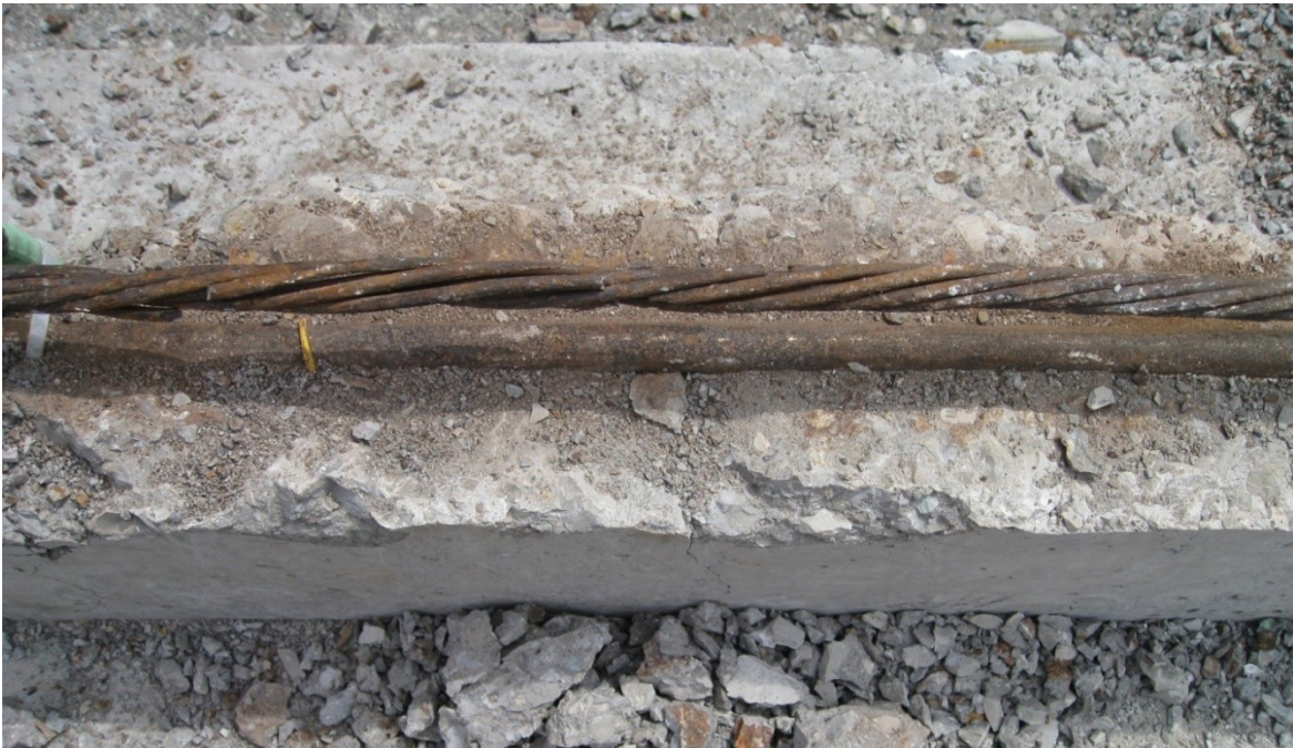
Figure 4-23 – Concrete strand interface above the strand
