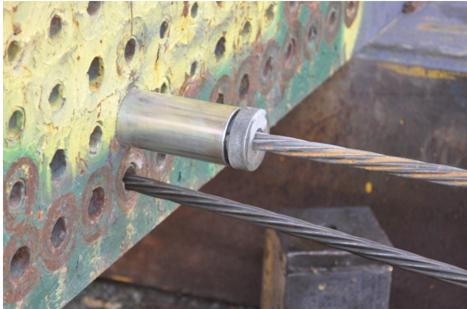
Figure 3-6 – Prestressing wedge anchor
