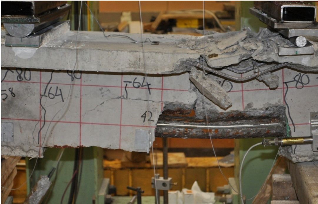
Figure 4-31 – Failure by concrete crushing of beam ST-2S-10%-NW-SC
