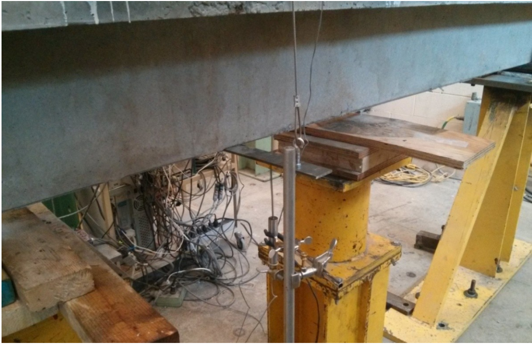
Figure 3-14 – Midspan deflection measurement by an external LVDT
