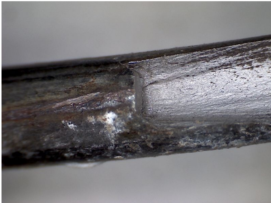
Figure 5-9 – Close up of the fracture surface of the wire shown in Figure 5-7 & Figure 5-8
