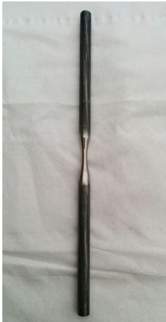
Figure 3-2 – Machined single wire specimens for fatigue testing
