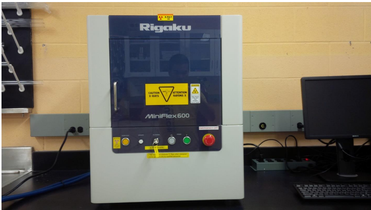
Figure 12 Benchtop XRD unit
