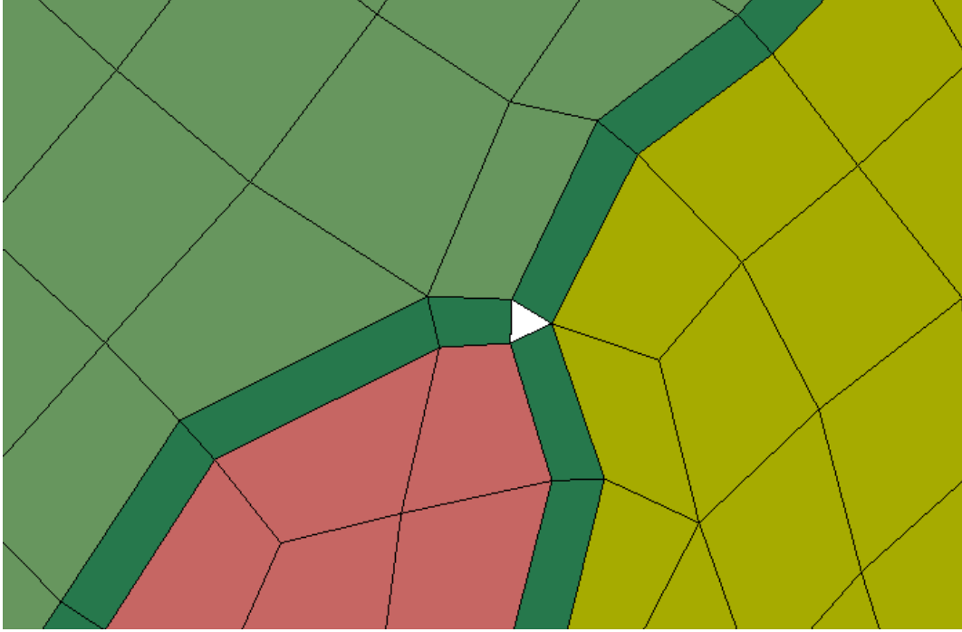
Figure 29: Hole located at triple point caused by creating grain boundary zones.
