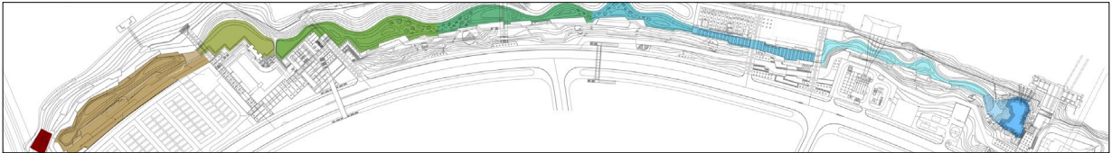
2.13 The stormwater management system for Houtan Park, illustrating different sets of wetlands for water purification and how they work together to treat the water during its journey through the park.
