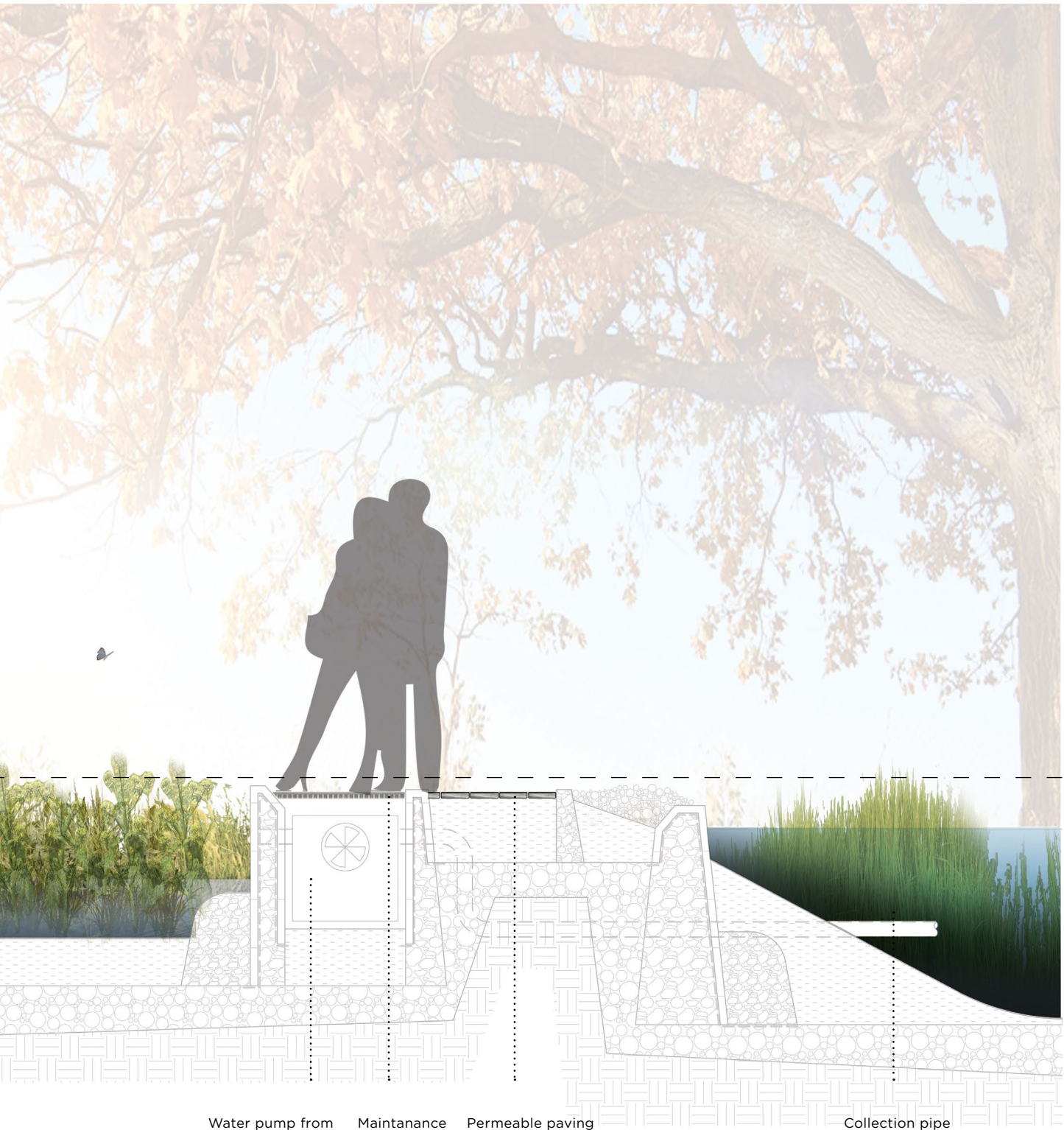
Water pump from pretreatment stage to water treatment basins
