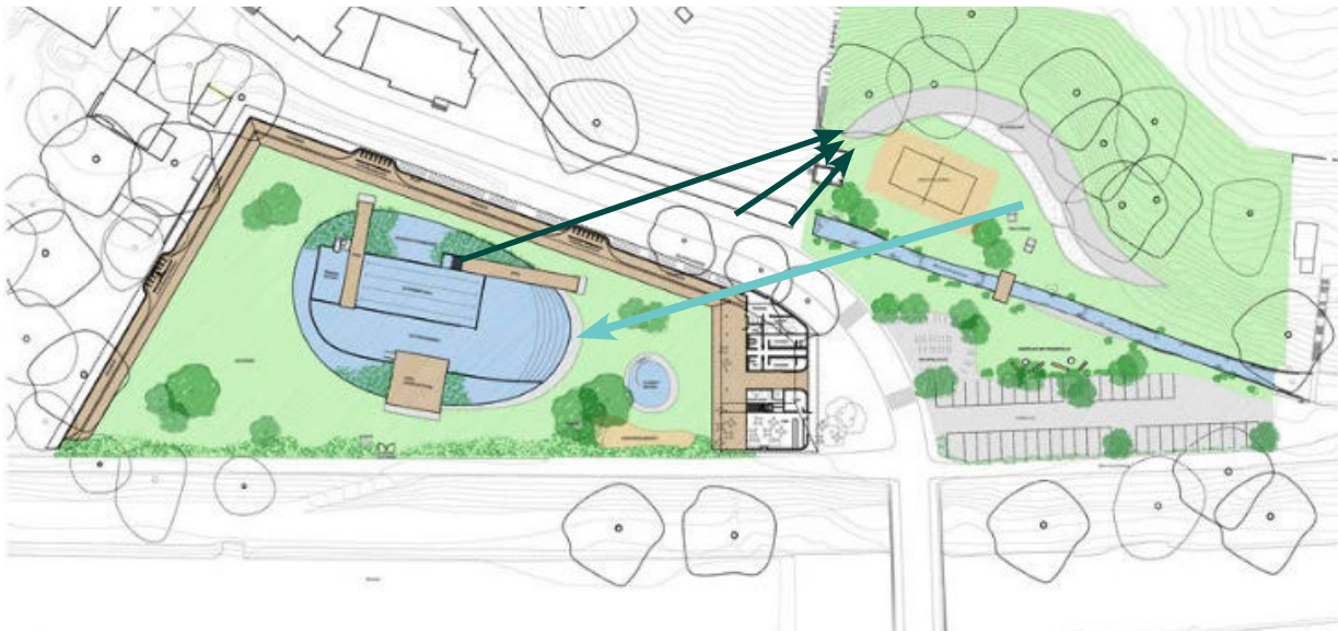
2.29 Bottom: diagrammatic plan showing the cycle of water, where green arrows indicate the flow of the contaminated water from the pool and street runoff and blue arrows show the flow of the treated water that runs from the natural filtration system on the slope of the hill.
