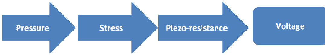
Figure 4-16 Principle of a piezoresistive pressure sensor
