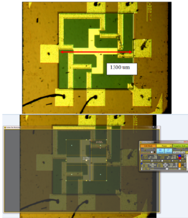
Figure 4-19 (a)Known Distance of MEMS of the MEMS Pressure Sensor, (b) Use of Golden Ratio to obtain the length of the diaphragm
