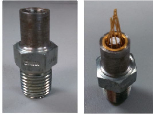
Figure 3-13. Steel case used as last interface with the Brake System (left), Steel case and TO Header subassembly (right).
