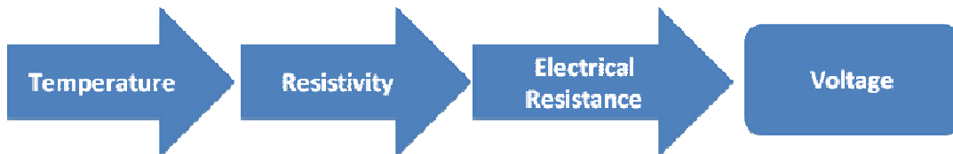
Figure 4-2 General transfer function of an RTD sensor.
