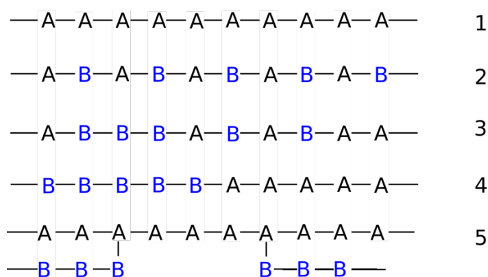
Figure 1: Different classes of copolymers. 1) Homo-polymer. 2) An alternating arrangement of A and B monomers, Alternating copolymer. 3) Random arrangement of monomers A and B in the
