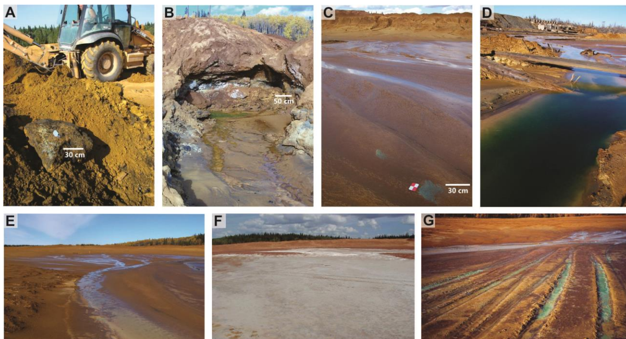
Figure 6-2: Photographs of the main areas where secondary sulfate minerals occurred. (A) A large block of melanterite-rich hardpan excavated from the Camp tailings; (B) the Seep Pool; note that in this photo the back wall had collapsed filling in the pool; (C) groundwater seepage from the Woods tailings dam along the Valley Seep with melanterite in the foreground; (D) a channel in the Valley Seep that collects all the groundwater seepage. Note the green colour of the water due to high concentrations of dissolved Fe(II). Photos (E) to (G) show Woods Seep (WS) in various seasons; (E) WS shortly after a rain event; (F) WS after a dry period in August with rozenite and melanterite blanketing the surface; (G) WS in October with melanterite precipitating in ATV tracks.
