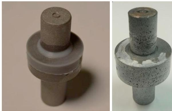
Figure 4-5: Pin and collar sample specimen (before cleaning [L], after machining with lathe [R])
