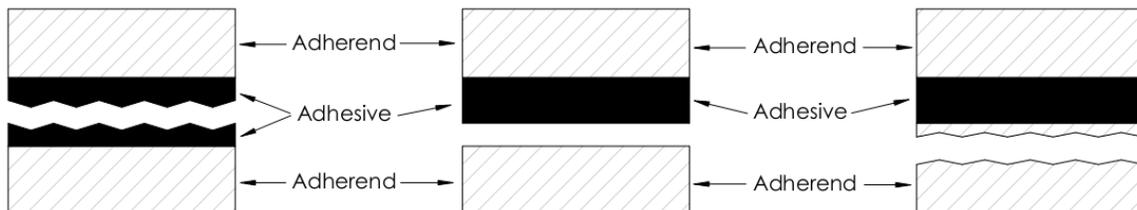
Figure 2-8: Joint failure types (cohesive [L], interfacial [M], structural [R])
