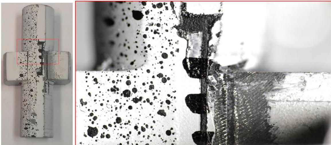
Figure 4-16: Sectioned sample (Schematic [T], Tested sample [B])
