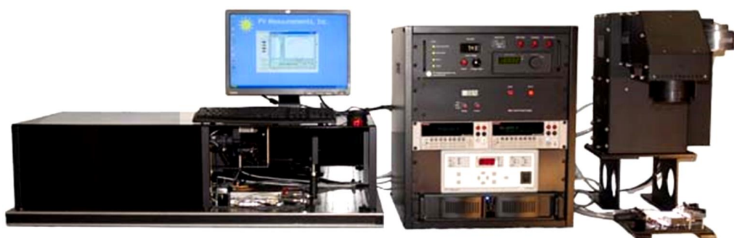
Figure 2.13 Photograph of a combined solar cell testing instrument from PV Measurements Inc. capable of current-voltage (I-V) characterisation with a solar simulator (IV-5, right) and a quantum efficiency measurement system (QEX-10, left).
