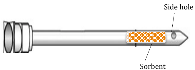
Figure 1.1. Schematic illustration of Shinwa needle trap
