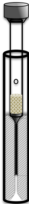
Figure 1.6. Schematic illustration of extended tip needle trap with designed narrow neck liner
