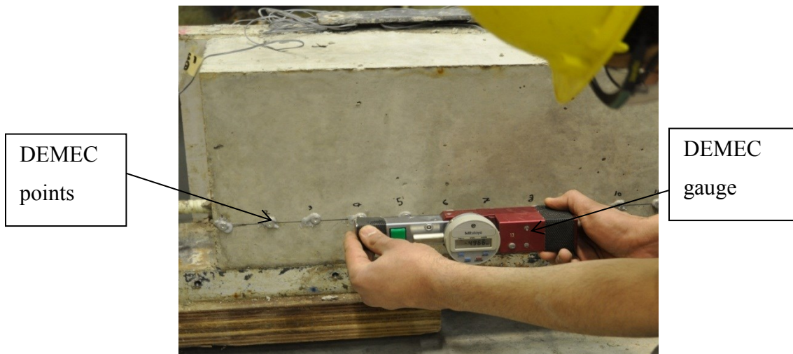
Figure 3.9: Concrete surface strains readings using the DEMEC gauge
