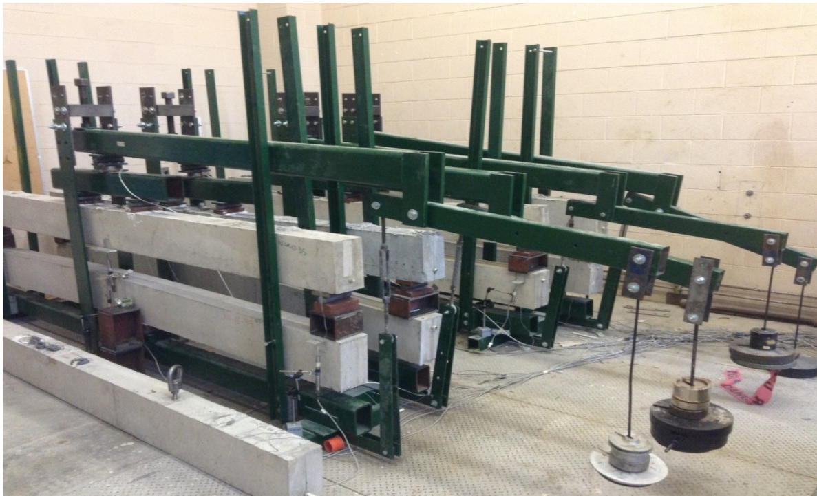
Figure 3.11 : Mechanical frames used for the beam sustained loading test.
