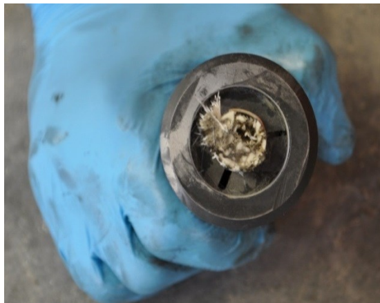
Figure 4.1: Failure mode of grpped GFRP bars in axial tension test
