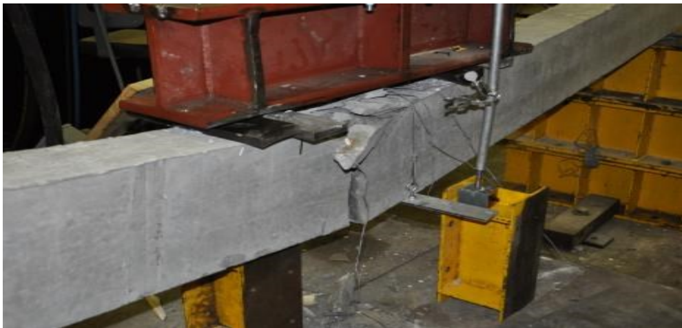
Figure 4.13: Failure mode for H40-16-0 beam
