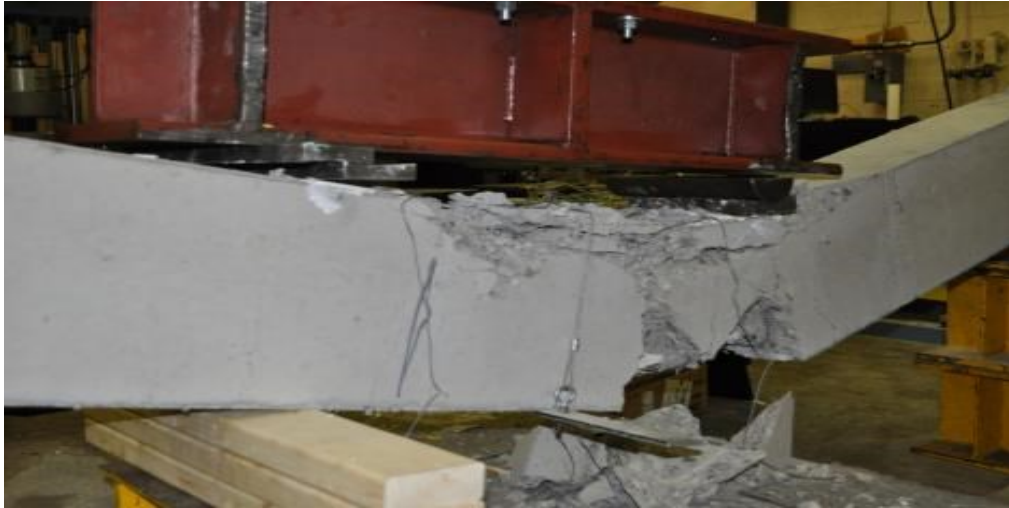
Figure 4.12: Failure mode for N0-16-0 beam
