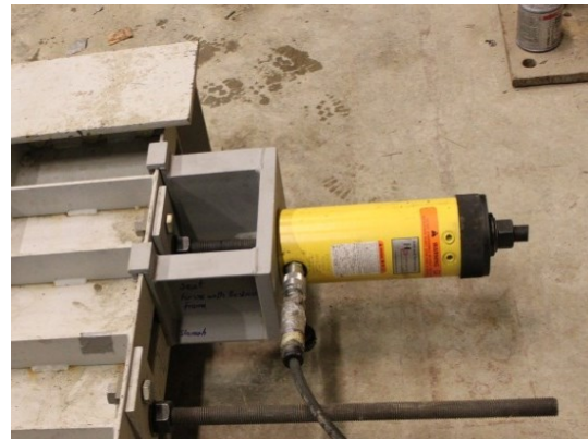
Jack installed on the threaded rod
