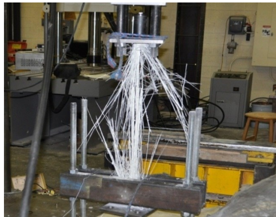
Figure 4.1: Failure mode of grpped GFRP bars in axial tension test
