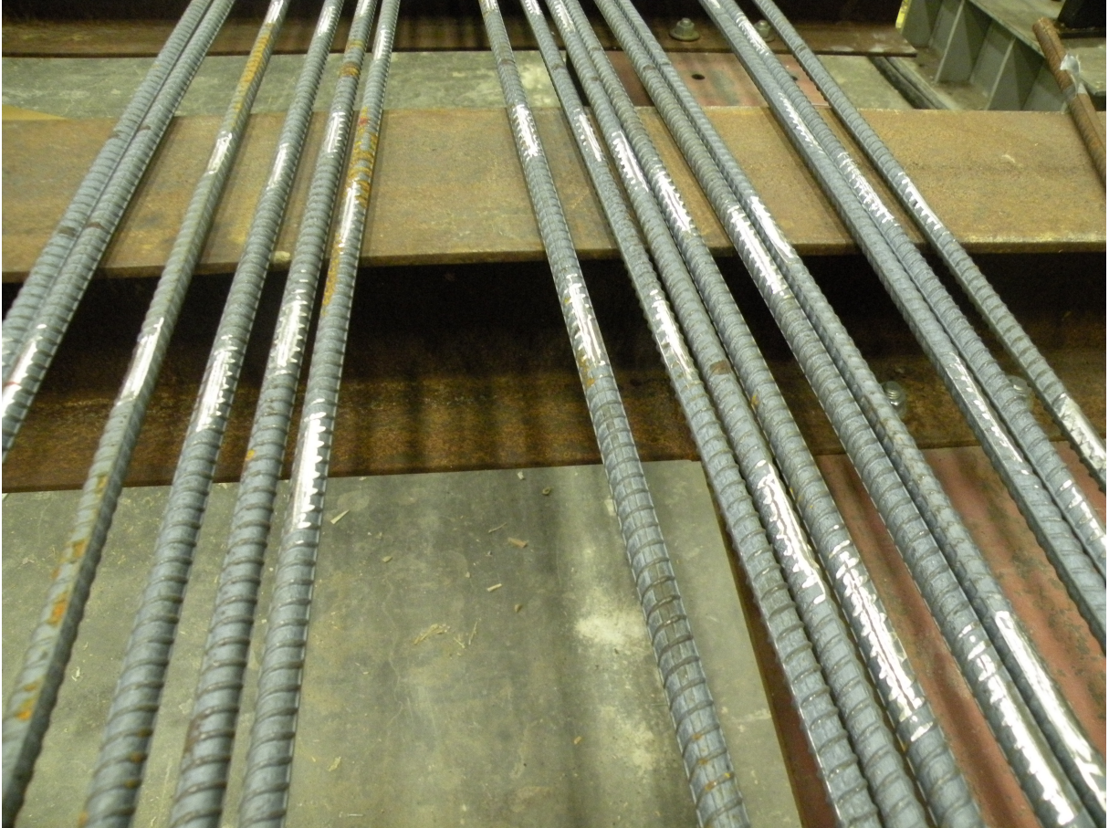
Figure 3.12: Strain Gauging of Flexural Reinforcement
