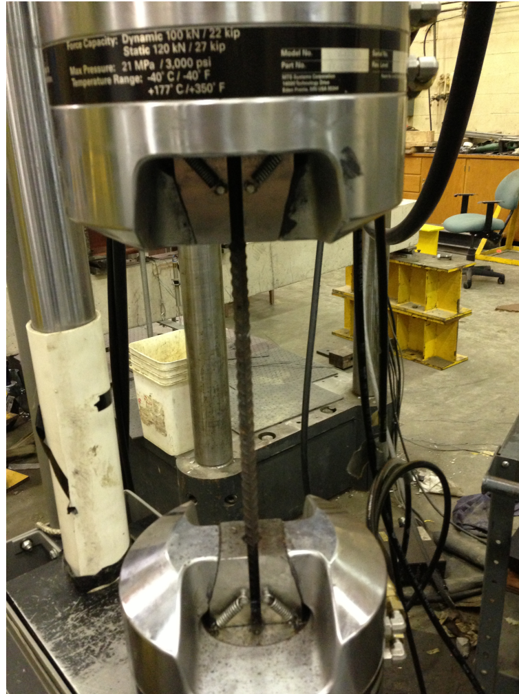
Figure 3.18: Tensile Testing of Flexural Reinforcement
