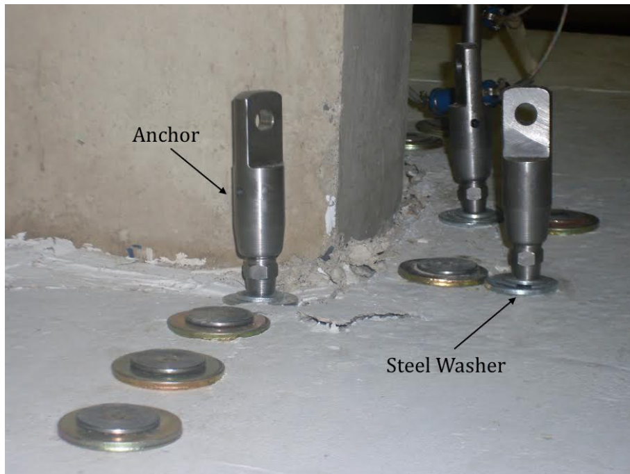
(c) Shear reinforcement on the slab
